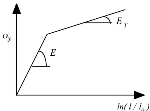
$$\begin{aligned} \nu &= 0,3 \\ E &= 200000 \text{ MPa} \\ E_T &= 2000 \text{ MPa} \\ \sigma_y &= 1000 \text{ MPa} \end{aligned}$$
