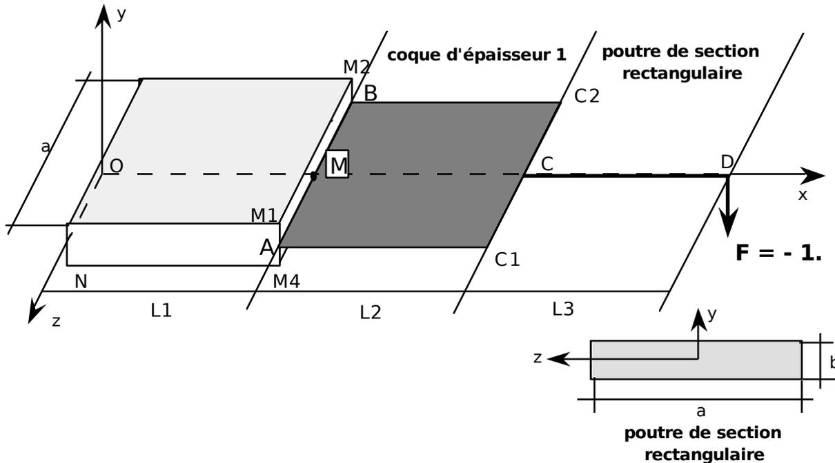
$$\begin{aligned} L1 &= L2 = L3 = 10 \text{ mm} \\ b &= 1 \text{ mm} \\ a &= 3 \text{ mm} \end{aligned}$$
