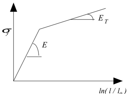
$$\begin{aligned} \nu &= 0.3 \\ \alpha &= 10^{-4} K^{-1} \\ \sigma_y &= 1000 \text{ MPa} \\ \text{à } T &= 20^\circ \text{ C} \\ E &= 250000 \text{ MPa} \\ E_T &= 2500 \text{ MPa} \\ \text{à } T &= 120^\circ \text{ C} \\ E &= 200000 \text{ MPa} \\ E_T &= 2000 \text{ MPa} \end{aligned}$$
